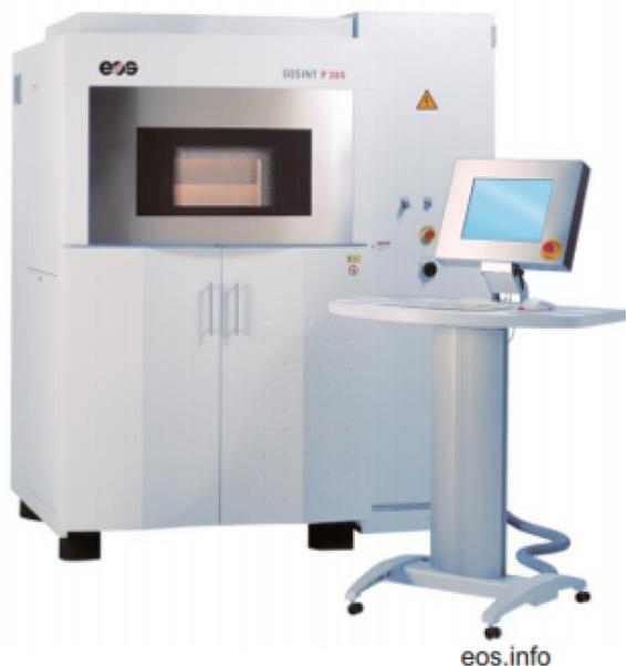
The EOS system can manufacture many different types of polyamide, including one polymer called PA12 (part of the PA 2000 series), a type of nylon. The EOS website lists PA12 series materials with tensile strengths that range from 48 to 54 MPa. However, due to the layer stacking manner in which parts are manufactured via SLS, part homogeneity and isotropy is a significant concern. To address this, the impact of part orientation of SLS parts on tensile strength was investigated.
