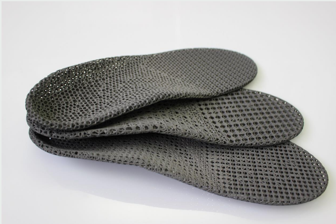
Image 9: Insoles with lattice structures printed with Ultrasim® TPU01, final part hardness 30-70 A depending on used lattice (Source: Forward AM).
