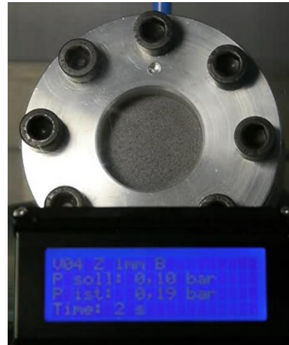
Test set-up for measuring burst pressure
