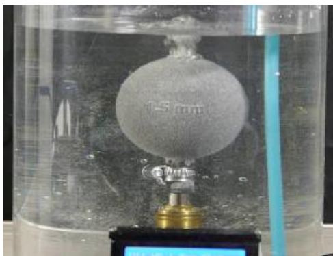
Air tightness of various geometries in Ultrasint® TPU 01
