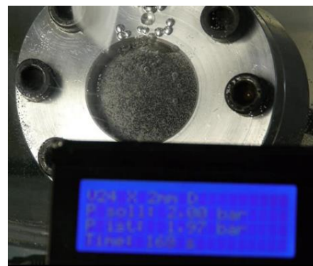
Test set-up for measuring air tightness
