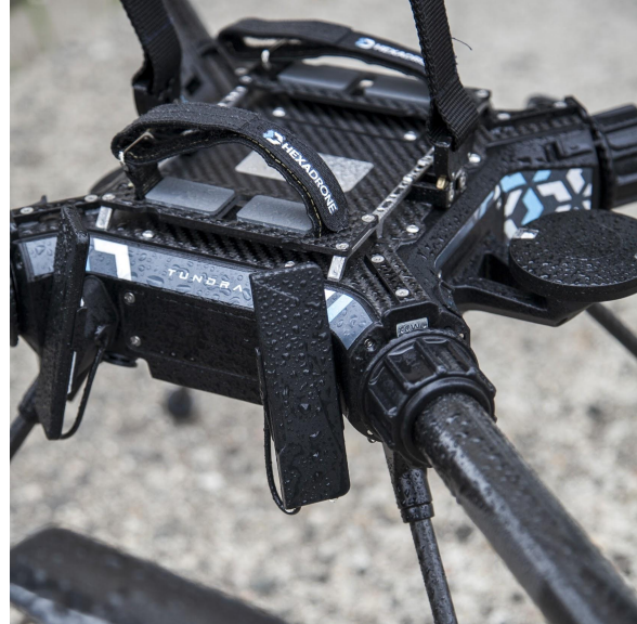
Tundra drone printed in Nylon PA12.
