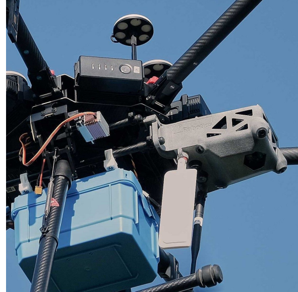
WeRobotics cargo drone with add on module printed in Nylon PA12.
