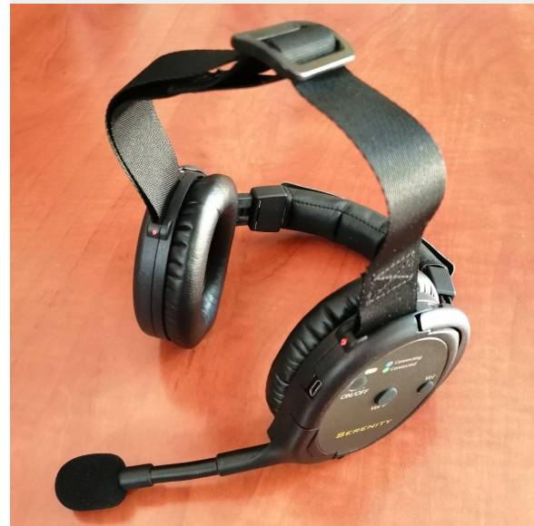
Overline-System's Headphone printed in Nylon PA12.
