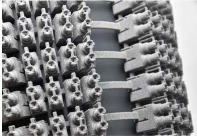
For versatility, we used MJF Ultrasint® TPU 01. Thanks to its flexibility, this material allows the belt to adapt to the user's back.
