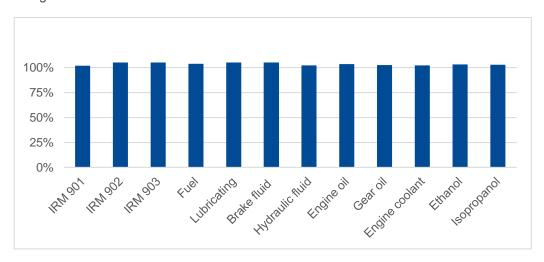
Change of volume of Ultrasint® TPU01 for exposure of chemicals
