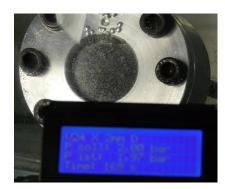
Test set-up for measuring air tightness
