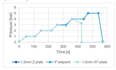
Air tightness of various geometries in Ultrasint® TPU01
