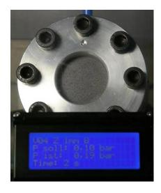
Test set-up for measuring burst pressure
